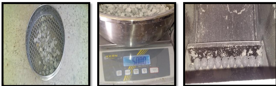
Figure III.26 Appareillage Los Angeles.
