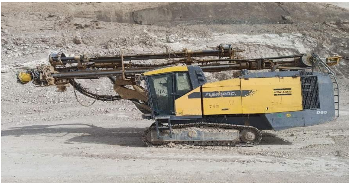
Figure II.12: Sondeuses de marques ATLAS-COPCO
