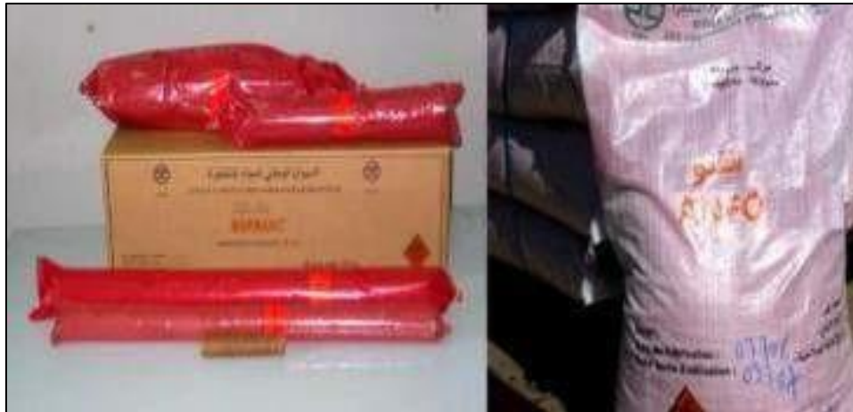
Figure II.13: Explosifs (Marmanite et Anfomil)
