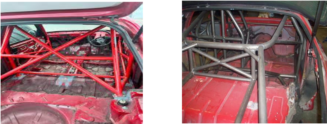
Figure 1.6: Example of application of truss system in the manufacturing of race cars
