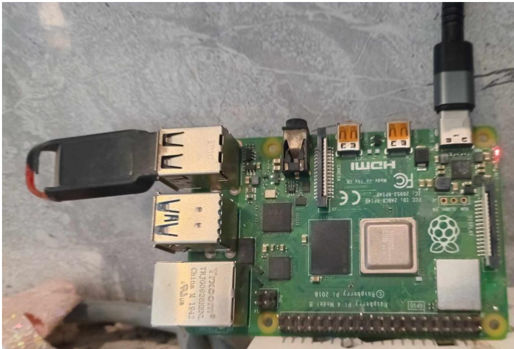
Figure III.17.: used Raspberry Pi 4 as the server for Home Assistant.
