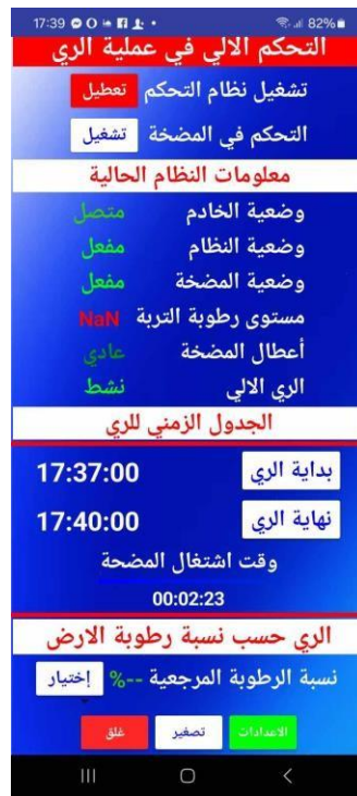
Figure III.25.: Third MQTT Android Application screen.
