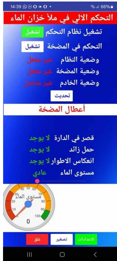
Figure III.26.: Fourth MQTT Android Application screen.
