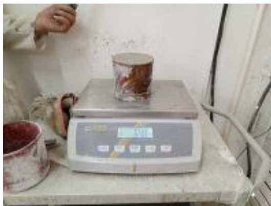
Figure 2. 11 Concrete density test
