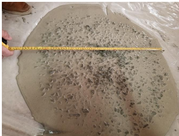
Figure 3. 1 Slump flow test on SCC
