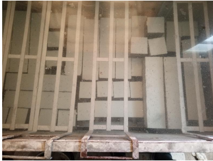
Figure 2. 7 Concrete samples curing in water
