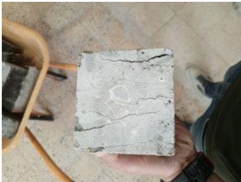
Figure 3. 4 Typical brittle failure of test specimen
