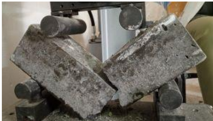
Figure 3. 10 Brittle failure of test specimen
