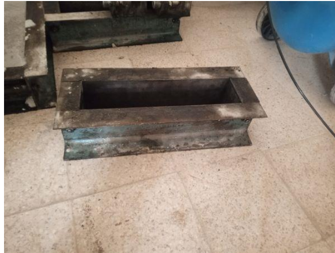
Figure 2. 9 Prismatic mould (10*10*40 cm 3 )
