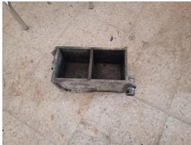
Figure 2. 8 Cubic mould (10*10*10 cm 3 )
