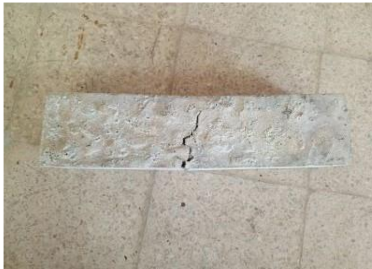
Figure 3. 11 Test specimen showing post failure integrity with increased fiber content
