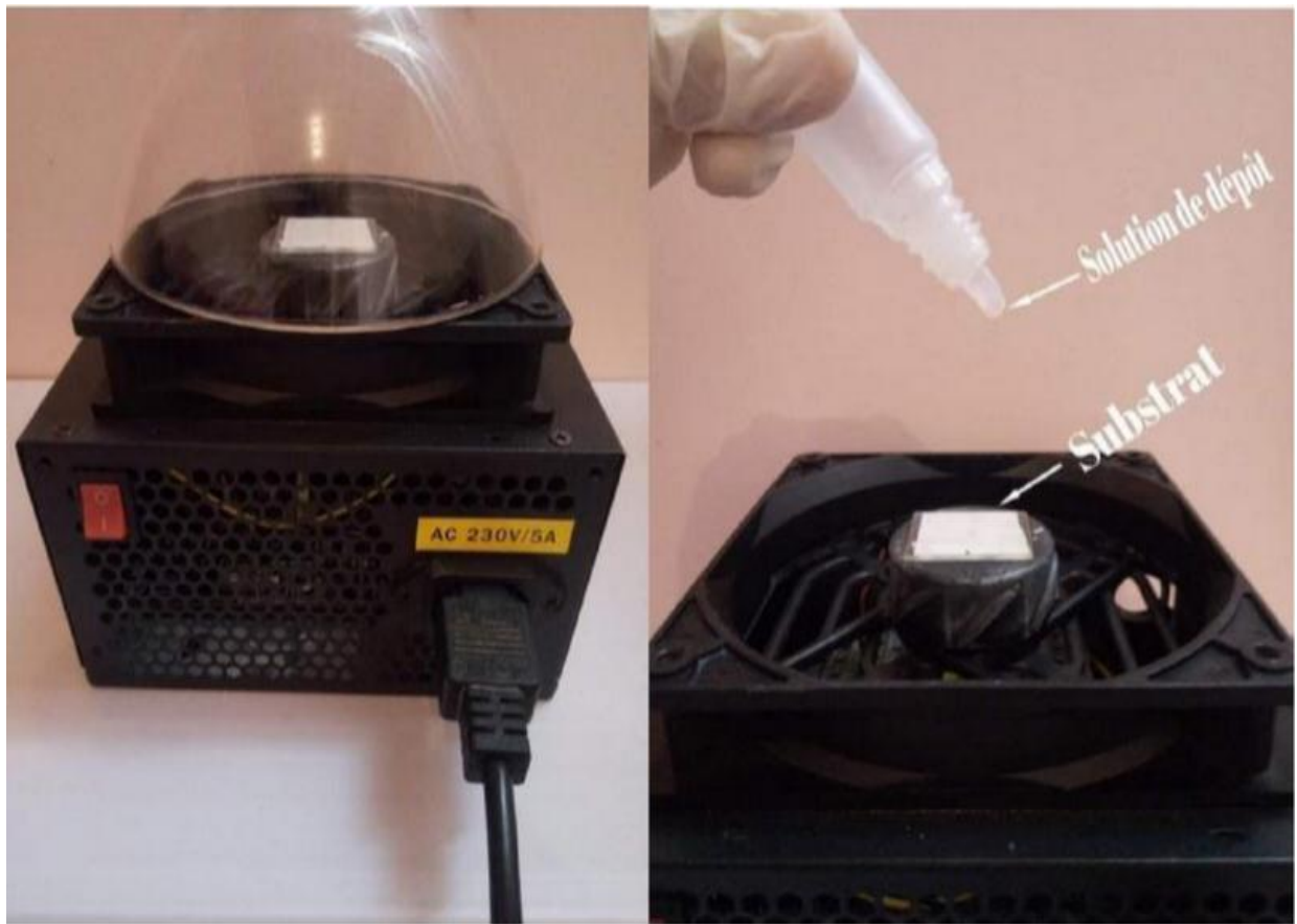
Figure II.2. Experimental spin coating device for the deposition of layers used at the Laboratory of Applied and Theoretical Physics, Echahid Cheikh Larbi Tebessi University - Tebessa.
