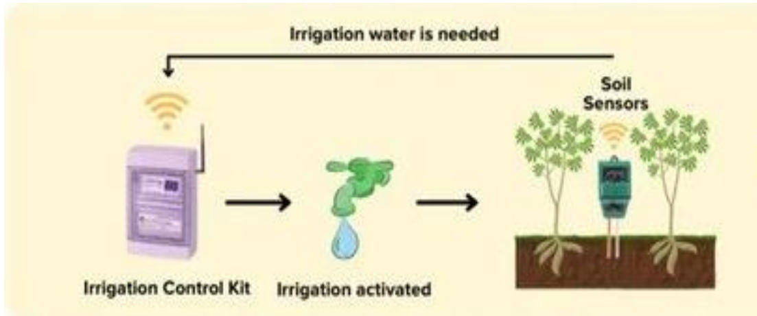
Figure 1.3: Example of AI application in soil management “Sensor Based Irrigation” [8]
