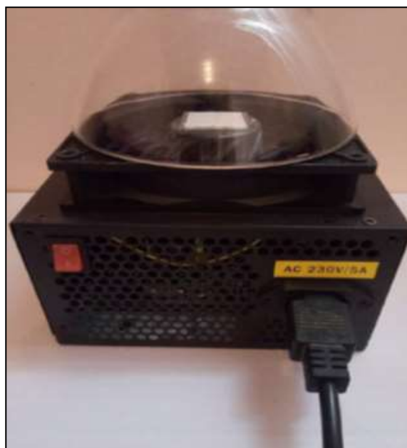
Figure.III.1. Experimental spin coating device for thin films.
