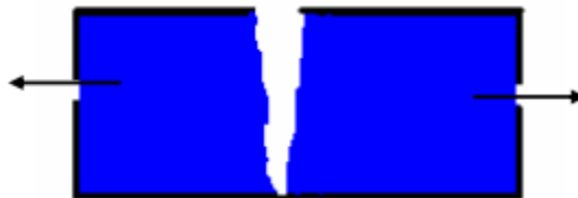
Figure I.5: corrosion sous contrainte.
