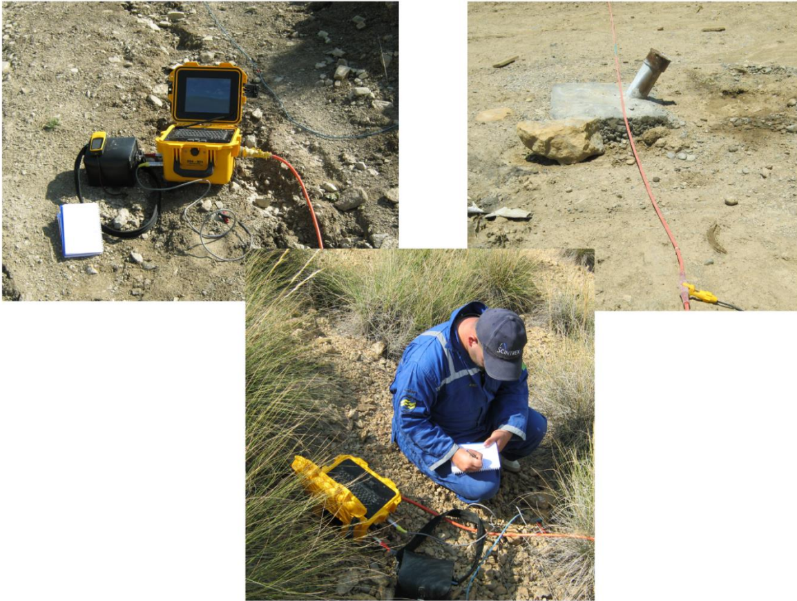
Figure 22: Summit X Stream Pro (DMT)
