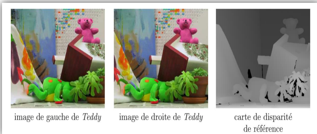
Figure [III.9] : Exemple de carte de disparité. (D. Scharstein and R. Szeliski - Middlebury Stereo Vision dataset).
