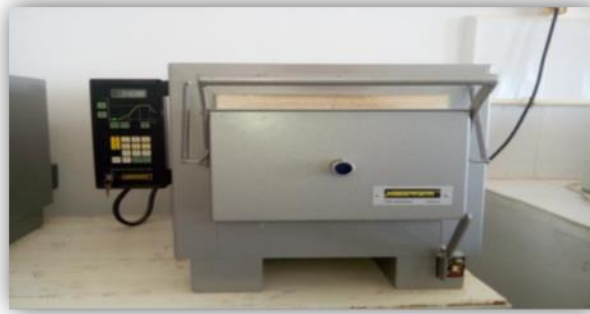
Figure II.13: Four de la marque NABERTHERM.
