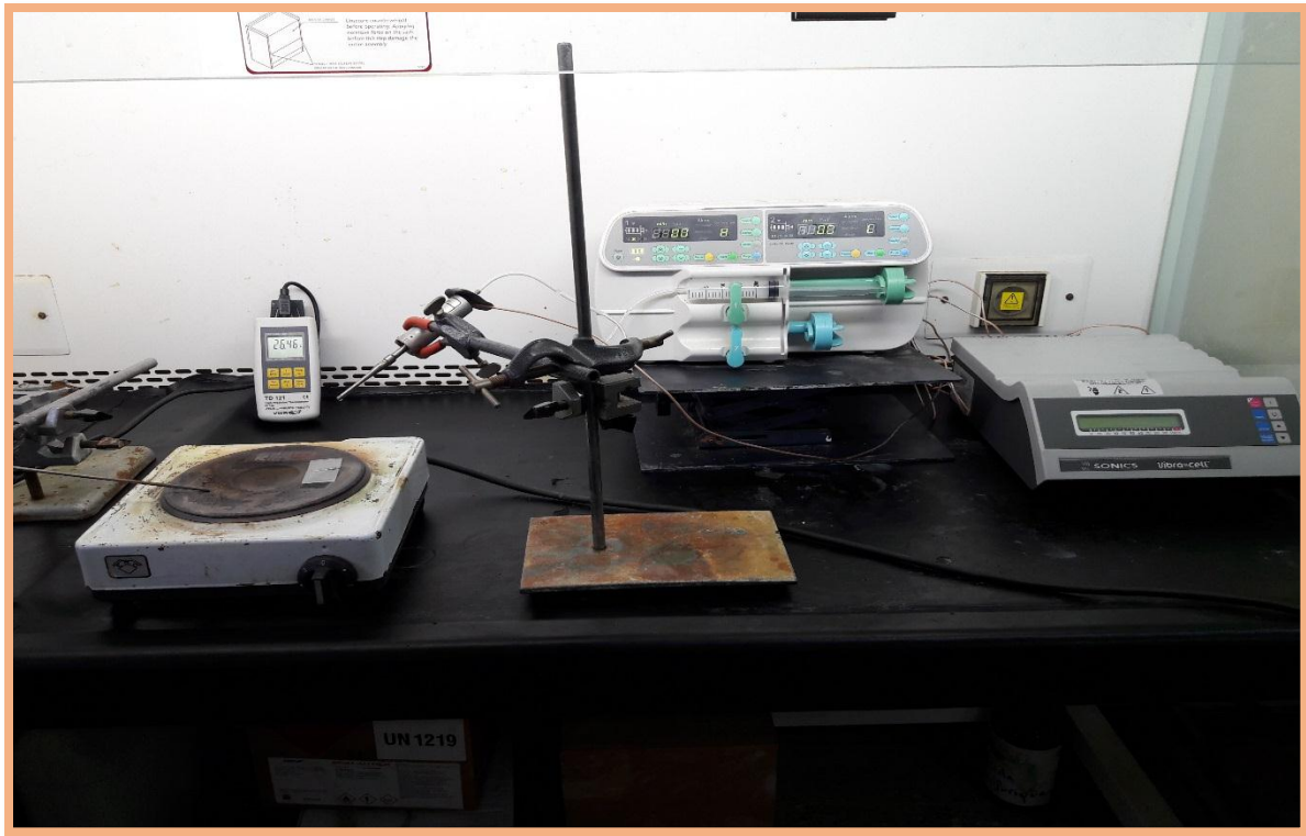
Figure II.5. Complete experimental devices of the ultrasonic spray pyrolysis technique.
