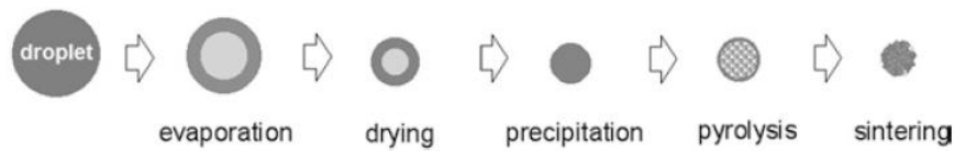
Figure III.4. Steps of powder production during the spray-pyrolysis [60].
