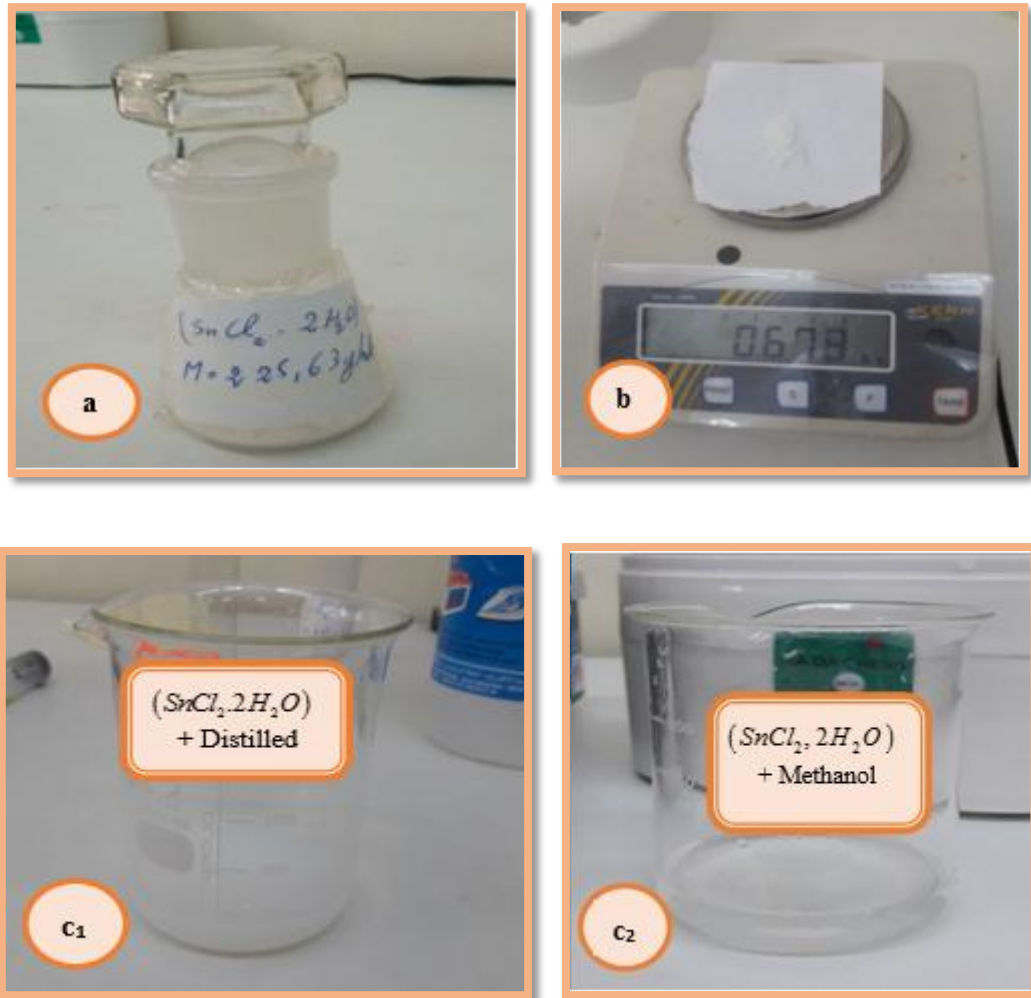
Figure II.4. Preparation of spraying solutions: a: TCD b: mass of TCD c 1 : (SnCl 2 .2H 2 O) +Distilled water c 2 : (SnCl 2 .2H 2 O) +Methanol.
