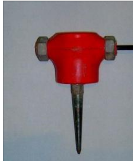
Figure I.24: Electromagnetic geophone, Picture of Wikipédia
