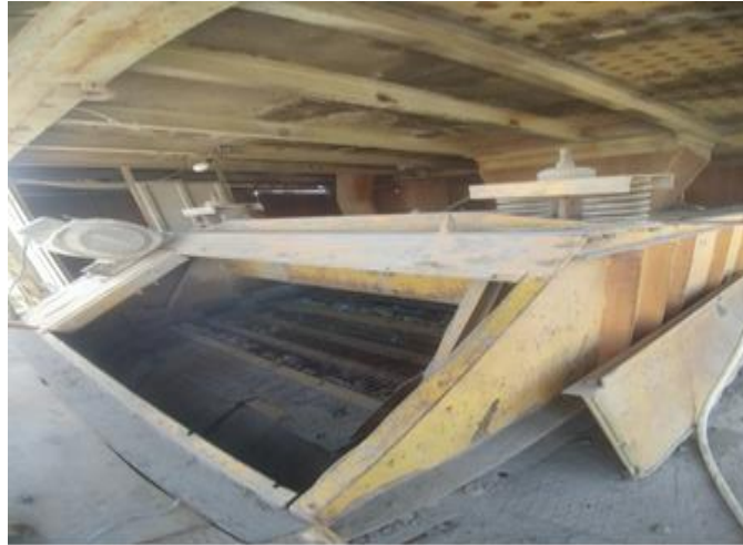
Figure I.13: Vue de crible vibrant de Kherzet Youcef, 2021
