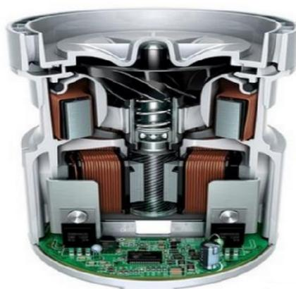
Figure 1. 11 Structure du MRV Dyson Digital Motor (DDM) [15]
