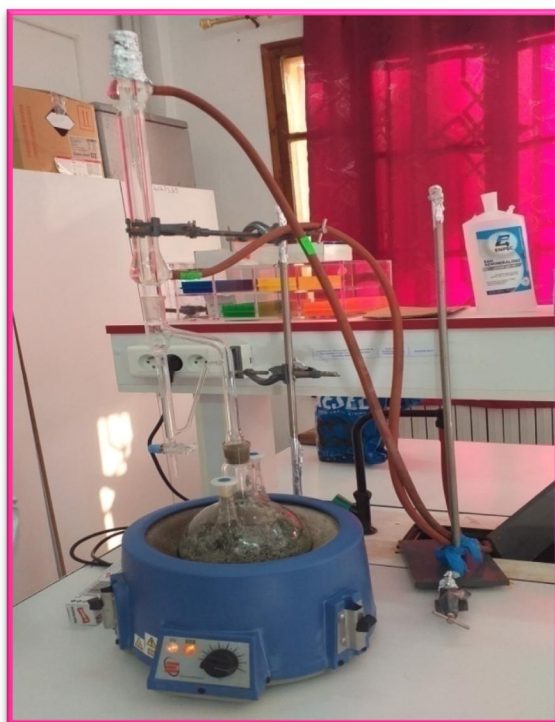
Figure 4: Montage d'hydro distillation
