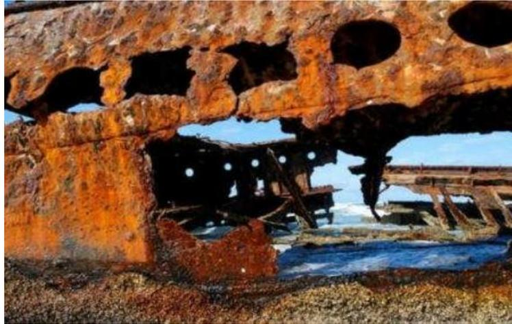
**Figure I.1 :** Corrosion uniforme [1].
