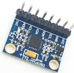
Figure V.10 Module Gyroscope MPU6050.
