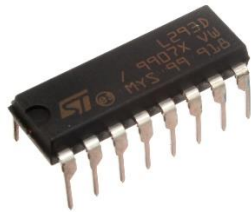
Figure V.15 Le circuit L293D [37].
