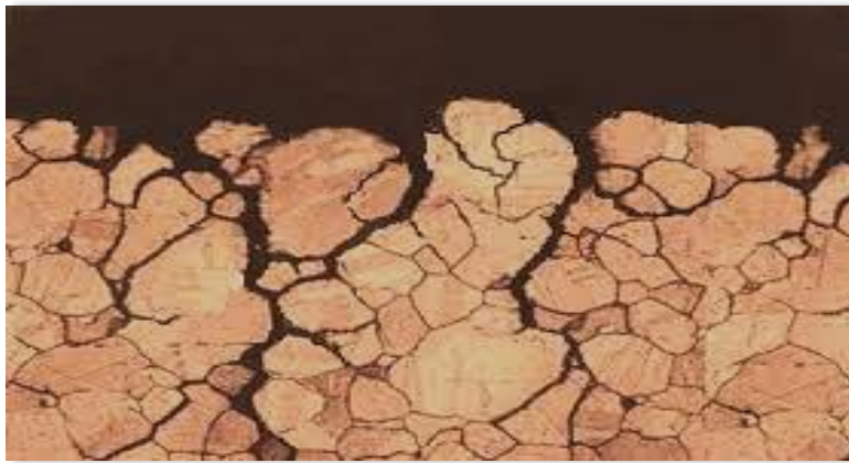
Figure I.6 : corrosion sous contrainte (C.S.C).
