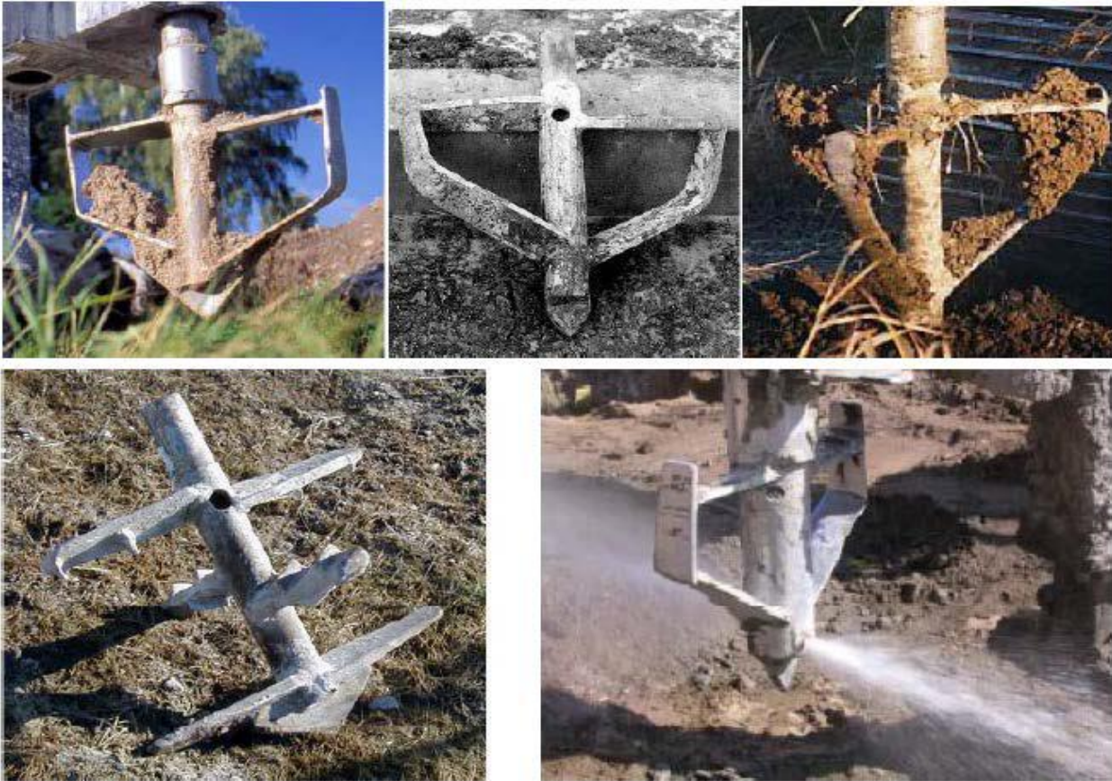
Figure 2.1 Example of simple rotary tools. Nordic dry mixing tools: a) standard, b) modified (Larsson, 2005)
