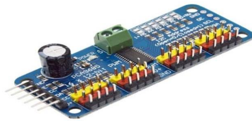
Figure 2. 3: Driver card PCA 9685 [17]
