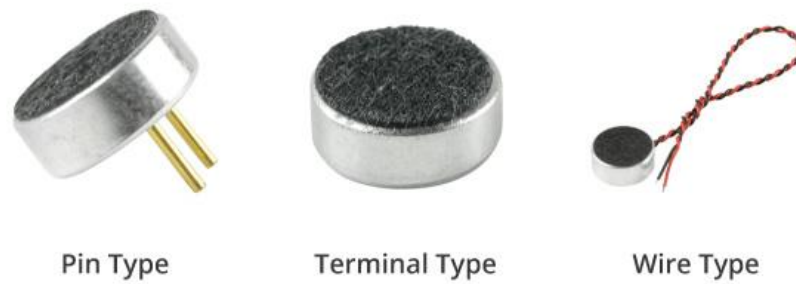
Figure III.9: Electret Condenser Microphone Mounting Types
