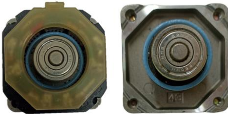
Figure III.14: Photo of normal bearing inside the motor
