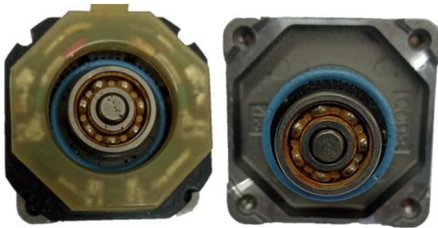
Figure III.16: Photo of a full rusty bearing inside the motor
