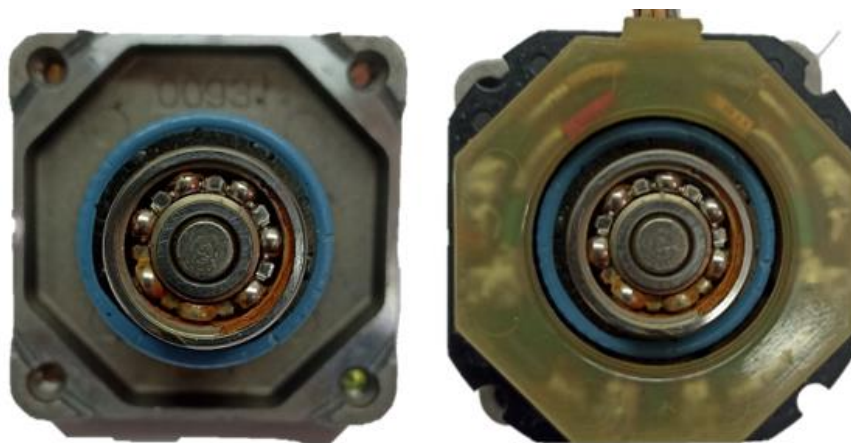
Figure III.23: Photo of a rusty spot bearing inside the motor
