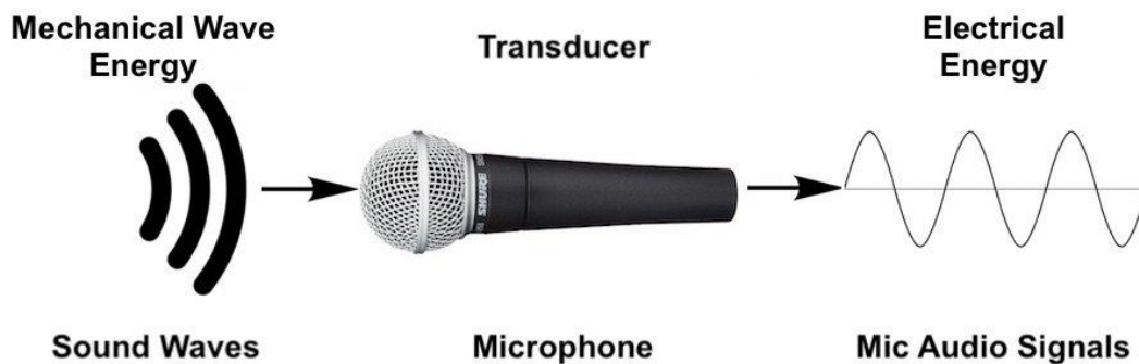
Figure III.6: Principal of mic
