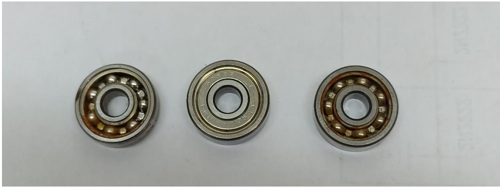
Figure III.13: Photo of different bearings (rusty spot, normal, full rusty)
