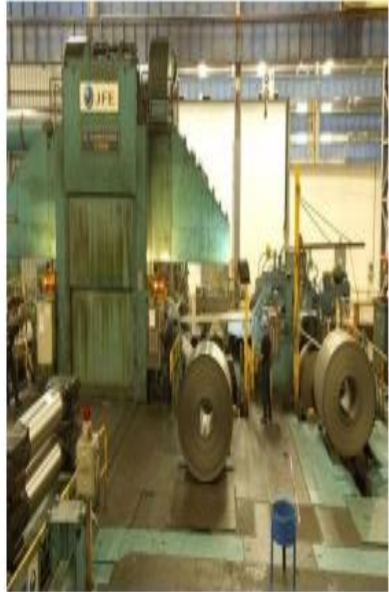
Figure II.3: Train de laminage [16].
