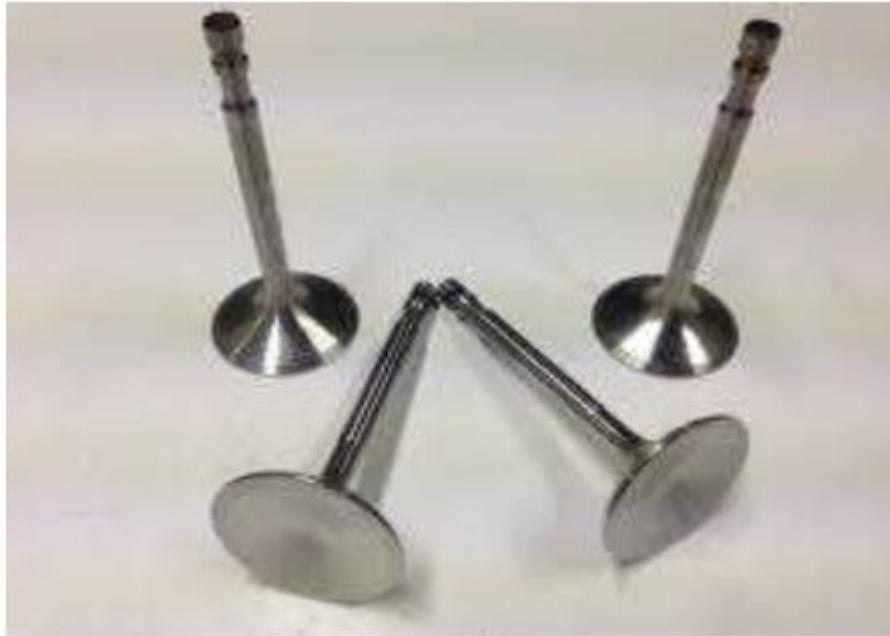
**Figure 1.9** Les soupapes
