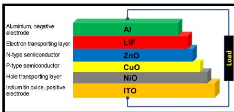
Figure I. 8: Representation of \text{Cu}_2\text{O} / \text{NiO} heterojunction solar cell [7].
