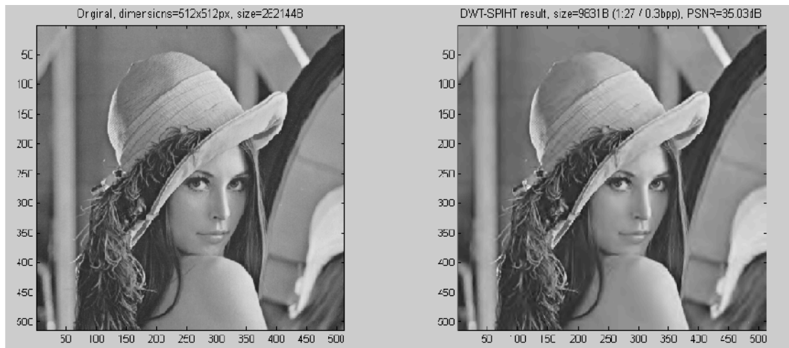
Figure 3.9 Lena image compression result at 0.3bpp
