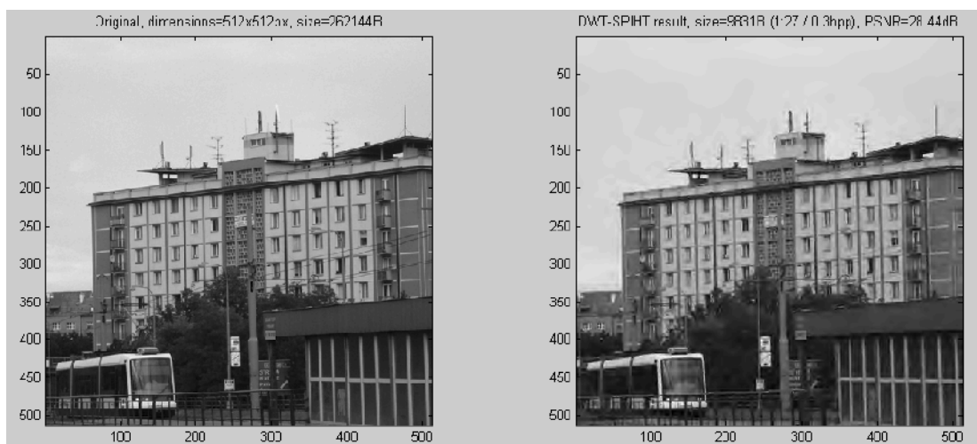
Figure 3.11 City image compression result at 0.3bpp
