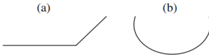
Figure II- 1: a) linear interpolation b) circular interpolation
