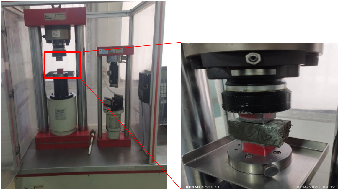
Figure II.13: Machine d'essai de compression
