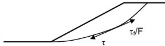
Figure 1 : Limit Equilibrium: Based on shear strength (Total or Effective stress approach).
