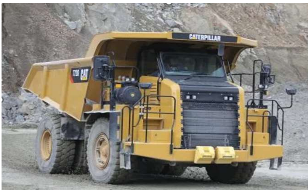
Figure III.9: Camion Caterpillar 770G
