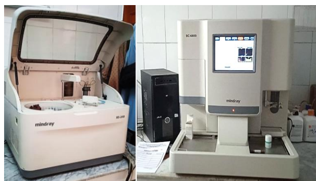
Figure15: Automated hematology analyzer (Mindray, BC-6800) (a), and automated clinical biochemical analyzer (Mindray, BS-240 pro) (b).
