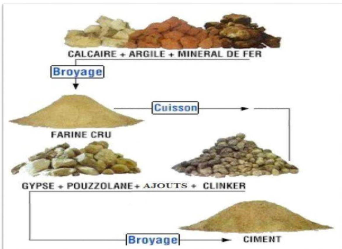
Figure 16: cycle de fabrication de ciment
