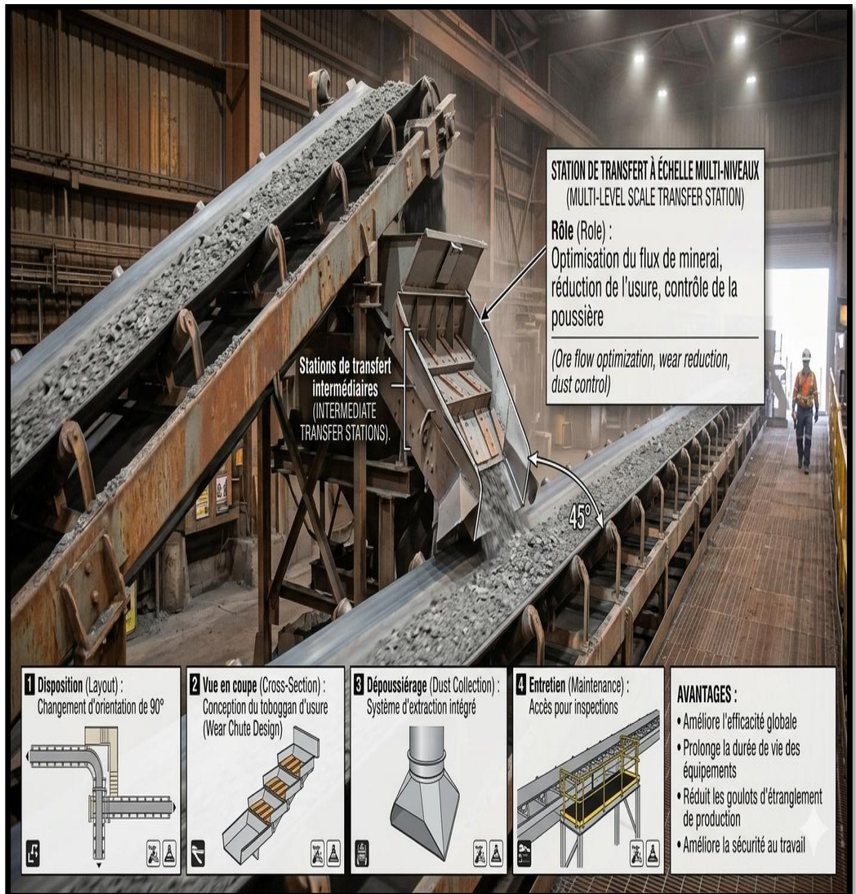
Figure II.26 Stations de transfert intermédiaires
