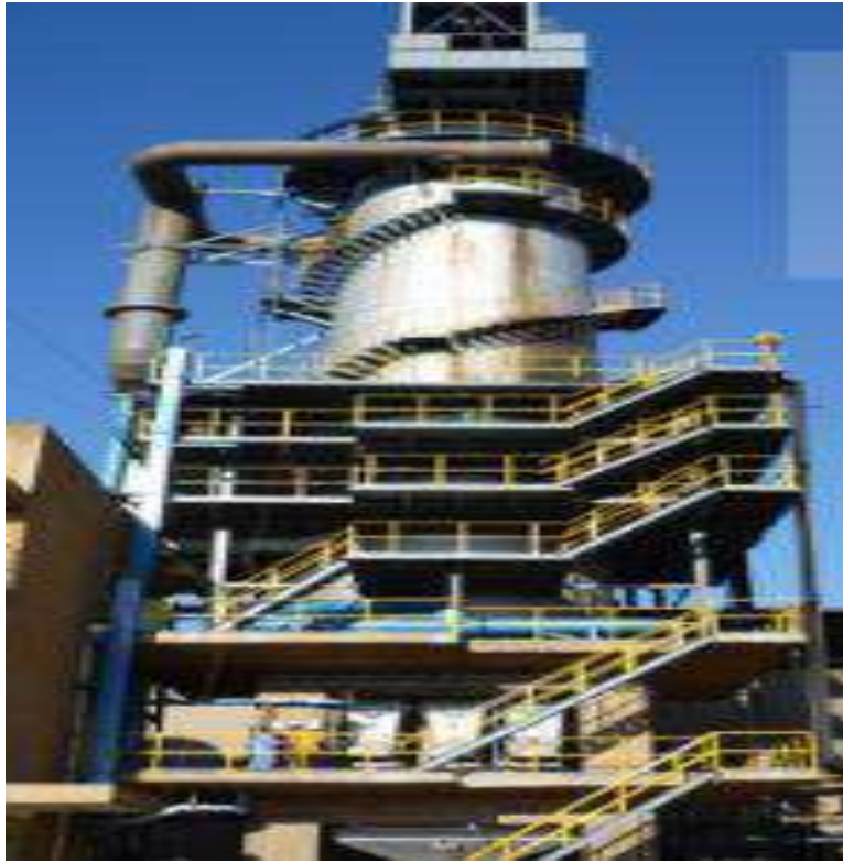
Figure 3.3: Four vertical ou four droit.
